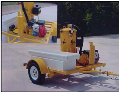
< Drum Vac-180 18 HP, gasoline powered vacuum unit mounted on a 2-wheeled trailer with storage tool box
